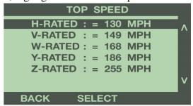
Note: Raising the top speed limiter is not recommended for vehicles equipped with load rated tires. Serious damage or injuries could occur. For more information on the Top Speed Limiter option, see Programming Features explanation in Section 4.
