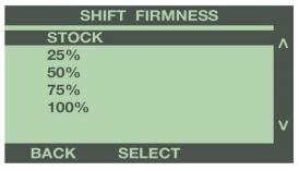
**PER GEAR SHIFT FIRMNESS:** Use the buttons to the right of the screen to scroll up or down, and highlight the gear change to adjust.
