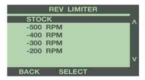
For more information on Engine Rev Limiter option, see Programming Feature explanation in Section 4.
