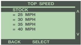
Some applications allow the top speed limiter to be lowered from the factory setting. On vehicles with this option, the initial top speed settings that appear on the programmer will LOWER the top speed from 25 to 75 MPH. Selecting one of these options will keep the vehicle from exceeding the selected speed.
