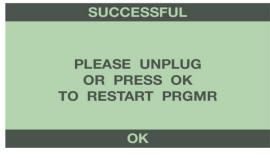
It is now safe to unplug the programmer from the vehicle and start the engine. Make sure the "Check Engine" light on the instrument cluster goes out (If it stays on or flashes, read out the DTC's, and contact Hypertech tech support). Warm up the engine and make sure it is running smoothly.
