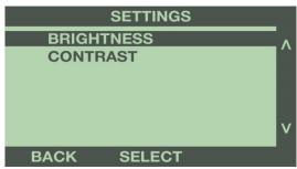
Use the buttons to the right of the screen to adjust the brightness or contrast of the display screen, from 1 to 10. Press the 'Back' button to return to the previous menu.
