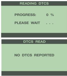
If the vehicle has any DTC's, the programmer will display the number of DTC's reported from the vehicle's computer. You can review the DTC's by pressing the 'Show' button. Before the programming process can begin, all DTC's must be cleared. To clear any DTC's, press the 'Clear' button. For more information on this feature, see the DTC section. Once the DTC's are cleared, the programmer will proceed to Reading Vehicle.
