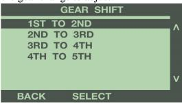
Press the 'Select' button, then use the buttons to the right of the screen to scroll up or down, and highlight the percentage to increase or decrease the shift firmness. Press 'Select' to save the chosen value.
